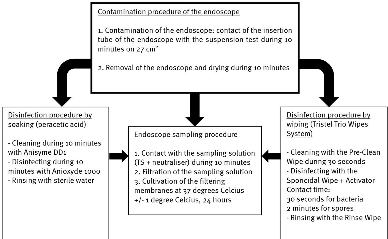
Figure I: Procedures and set-up of the contamination, disinfection and sampling tests.
