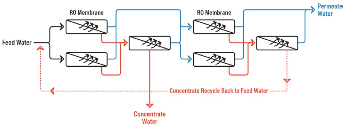
**Figure 7:** Visual representation of the 1 pass and 2 pass RO systems (<https://puretecwater.com>)
