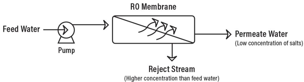
Figure 2: A simplified representation of the RO system (<https://puretecwater.com>)
