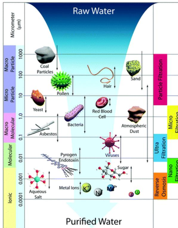
Figure 3: Membrane filtration spectrum (Lee et al., 2016)
