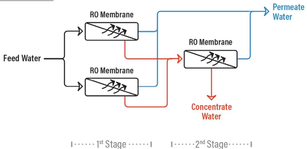
**Figure 6:** Visual representation of the 1 stage and 2 stage RO systems (<https://puretecwater.com>)
