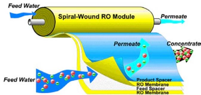
Figure 4: Spiral-wound RO membrane (<http://www.sapphire-water.ca>)
