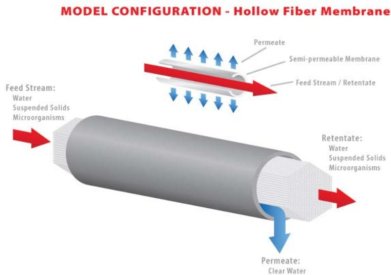
Figure 5: Hollow-fibre RO membrane (<http://synderfiltration.com>)
