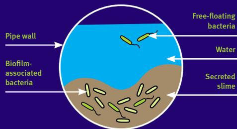
**Figure 3. Biofilm forming inside a water pipe**
